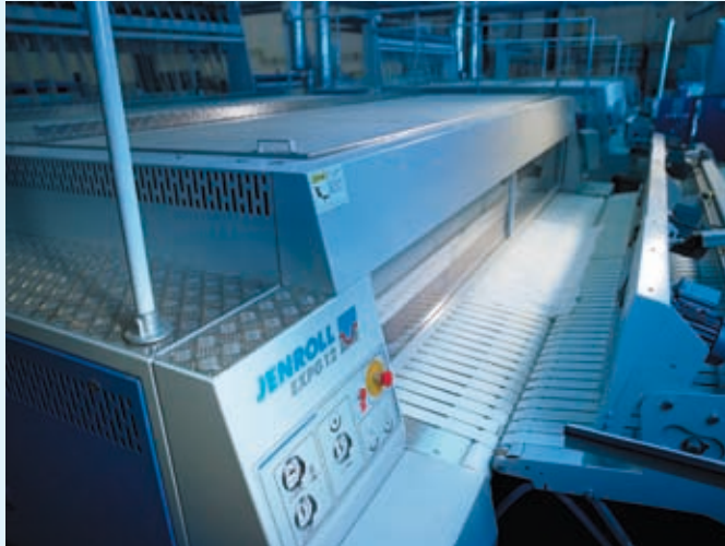
Jenroll EXPG with 2 rollers, 1200 mm diameter each.
